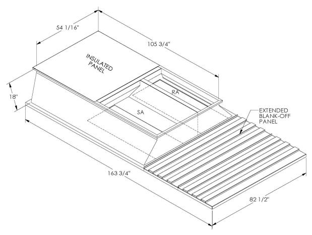
ONE PIECE WELDED CONSTRUCTION
