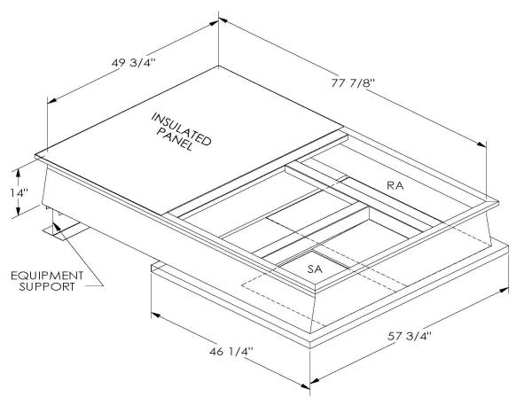
ONE PIECE WELDED CONSTRUCTION
