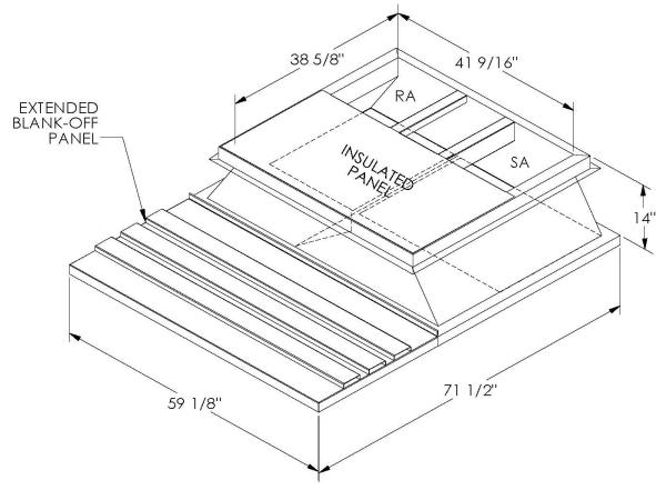
ONE PIECE WELDED CONSTRUCTION
