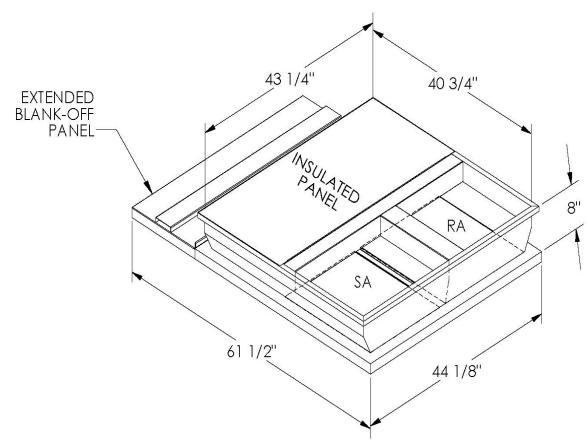
ONE PIECE WELDED CONSTRUCTION
