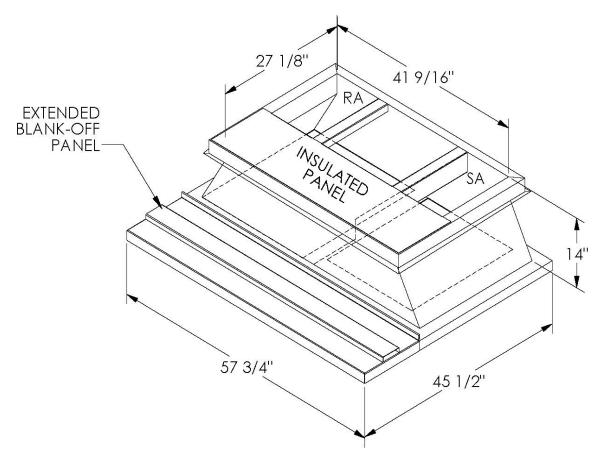
ONE PIECE WELDED CONSTRUCTION
