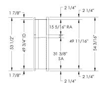
$\ensuremath{^{\ast\ast}}$  New unit can sit on existing curb without adapter with overhang
