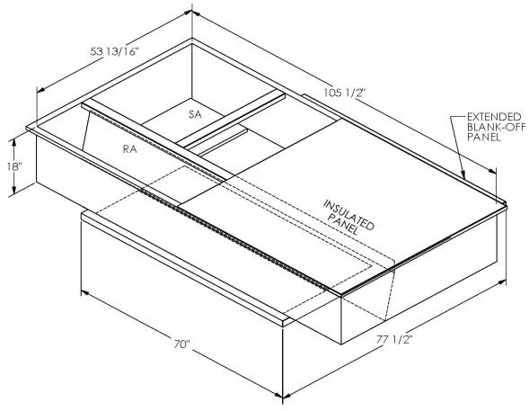
ONE PIECE WELDED CONSTRUCTION
