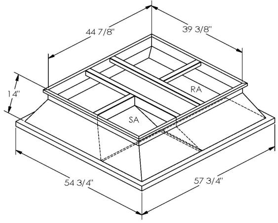
ONE PIECE WELDED CONSTRUCTION
